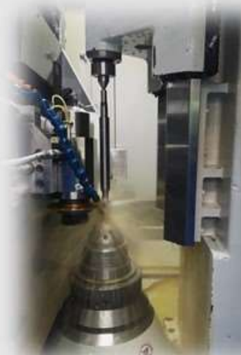
Richardon R200 CNC Thred –snails milling
